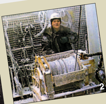
Air and hydraulic winches can offer constant tension for mooring and sea going applications.
