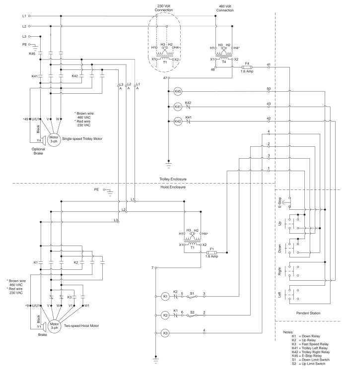
Single Speed, Three Phase Trolley with Emergency Stop and Dual Speed, Three Phase Hoist
