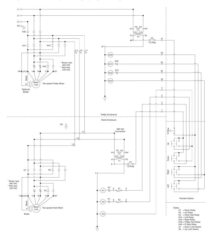
Dual Speed, Three Phase Trolley with Emergency Stop and Dual Speed, Three Phase Hoist
