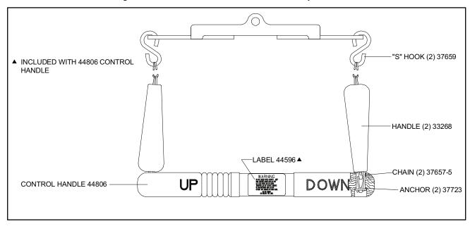
Figure 22. 40004–5 Pull Chain Control Assembly (MHP3443)
