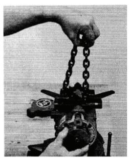
Figure 7. Installing Load Chain (MHP3428)
